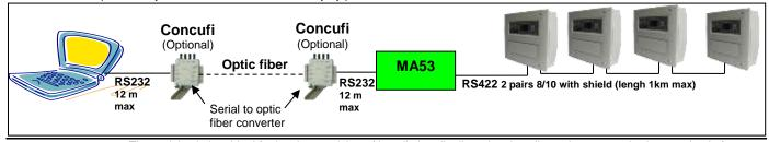
The serial solution, ideal for local supervision of installation distributed on low dimensions areas, is characterized of a single operating point (PC).
