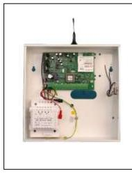
**GSM 31 GPRS:** GSM/GPRS communicator (with metal enclosure, GSM antenna and power supply). Can be used as accessory controlled by a control panel or used stand alone as alarm unit. It can be used as backup for telephone line in case of fault. Needs a SIM card. Allows to transfer general informations from the fire detection panel through GSM/GPRS messages (SMS).
