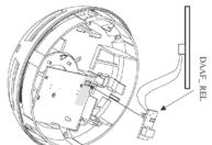
Base and detector connection for DAAF-INTER Optional board
