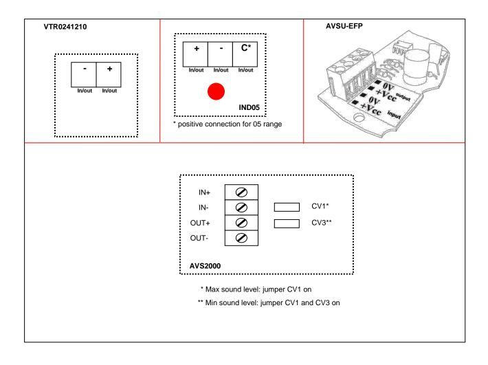
REFERENCE<br/>IND05DESCRIPTION<br/>Remote alarm indicator angle of vision = 180° (IND05E: water proof version)AVS2000/R<br/>AVSU EFPSounder piezo red color<br/>High powered piezoelectric sounder for outdoor, 114db @ 1m, IP65VTR0241210<br/>VTRSSOLElectromagnetic door release unit<br/>Floor support for magnet VTR0241210
