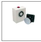
**VTR0241210 Electromagnetic door release unit:** Electromagnetic door holders mounted in a steel box + rotating equipped keeper-plate. It is designed to hold open fire or smoke stop doors, for convenience and then release automatically them in response to an emergency. The keeper plate is mounted on a rotating and shock-absorbing support for angles  $\leq$ 60°. Release push-button.
